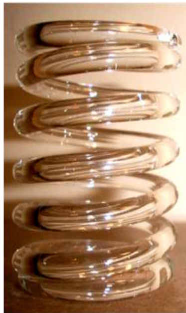
Figure 4.2. Spring sample used for creep-recovery experiment in the Parallel Plate Viscometer
