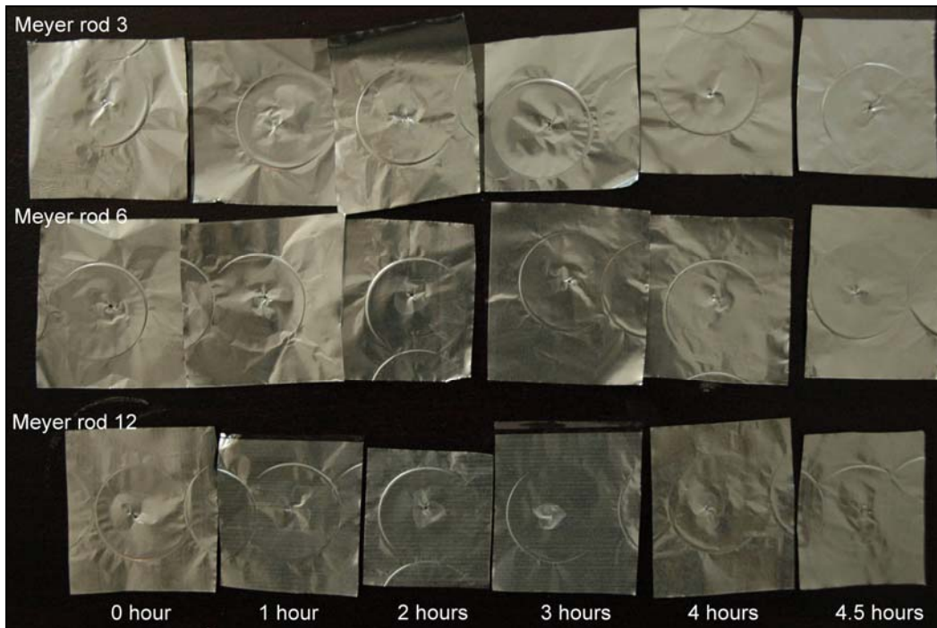
Figure 4.2: Delamination over time using ASTM probe from PET side
