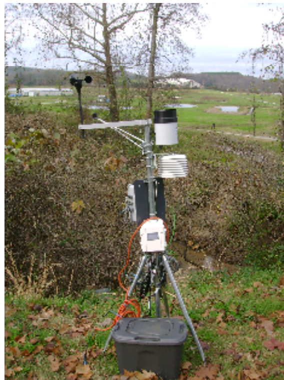
Figure 5. HOBO Onset U30 GSM data logger and weather station.
