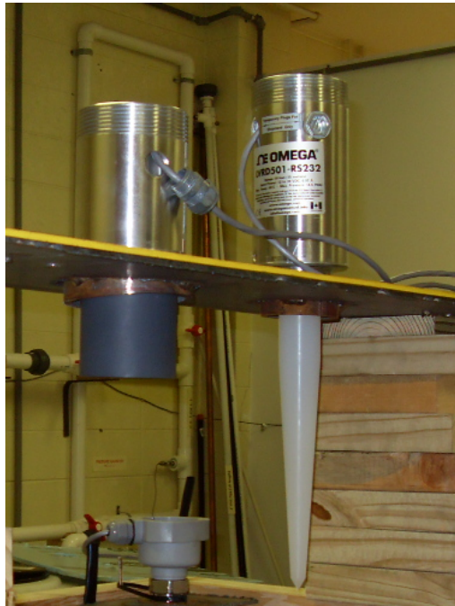
Figure 1. Ultrasonic transmitter (left) and radar level sensor (right).
