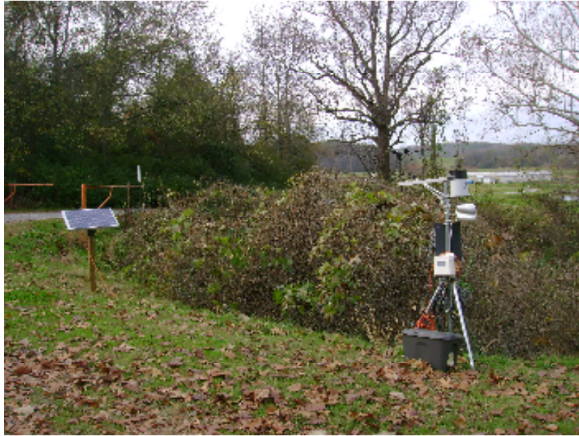
Figure 6. Weather and data logging station with solar panel.
