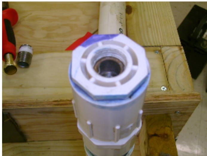
Figure 2. Pressure transducer inside protective fitting.
