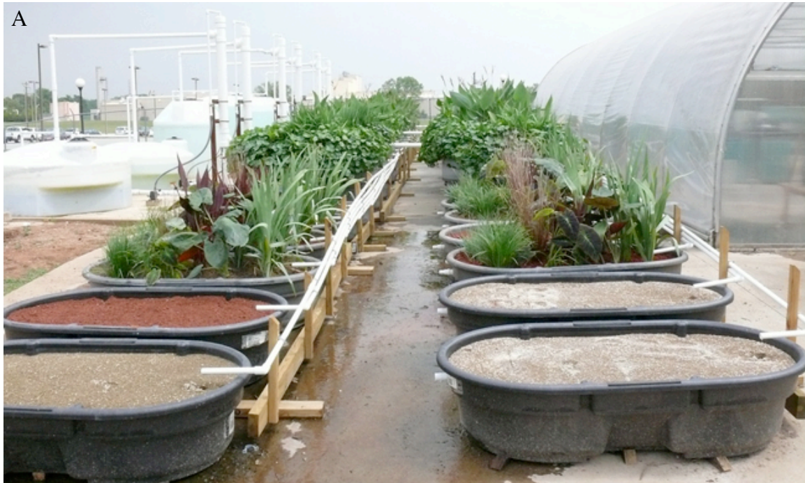
FIGURE S4.1. Mesocosm primary surface-flow to secondary subsurface-flow CWS in May 2007 (A) and August 2007 (B).
