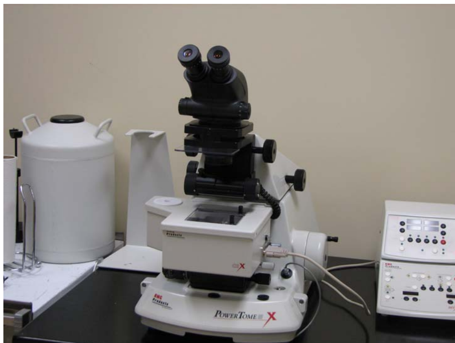
Fig. 2.8: Cryomicrotome utilized to cut thin specimens for observation under TEM
