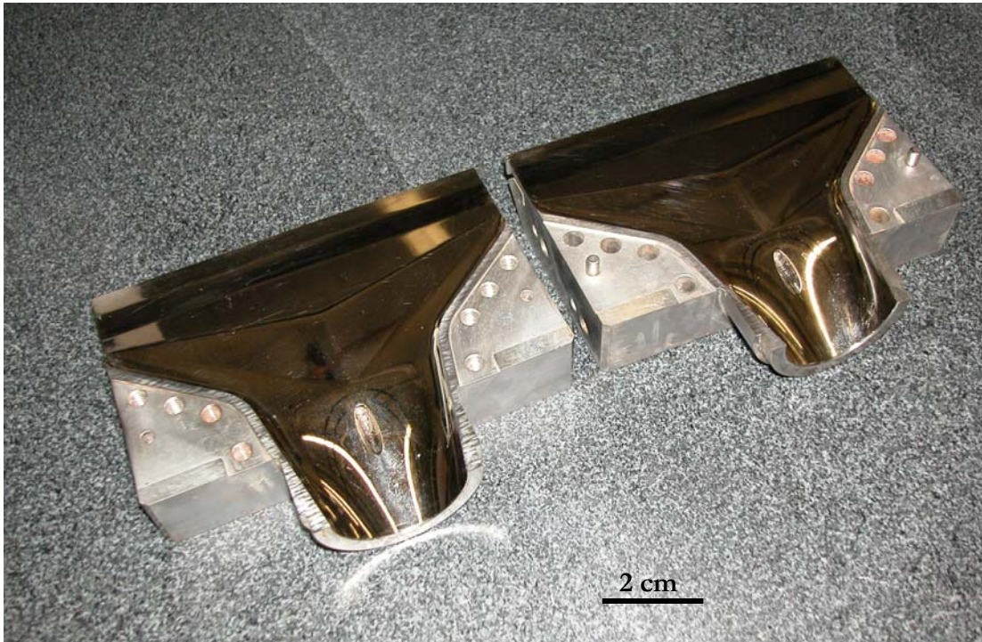
Fig. 2.4: Photo showing the faces of the coat-hanger die used in this study
