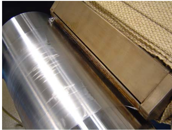
Fig. 2.1: CCB laboratory setup shown here in operation. Also seen is a closer view of the film exiting the die onto a chill roll
