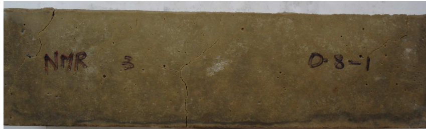
Soaked in 3 Molar KAc Solution and Blended Deicers with Li/K 0.8
