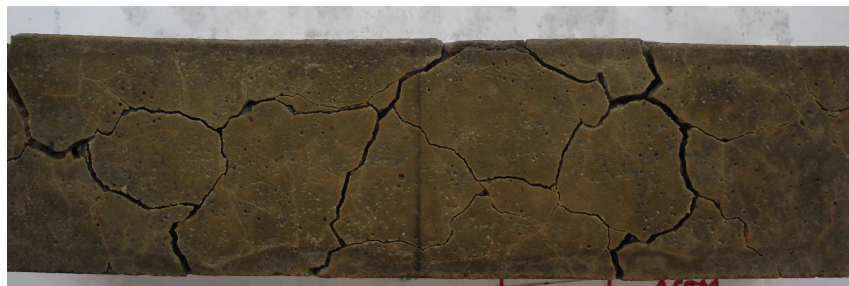
Soaked in 6.4 Molar KAc Solution and Blended Deicers with Li/K 0.2
