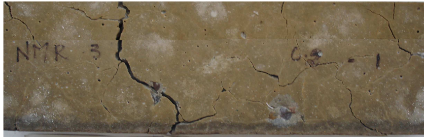
Soaked in 3 Molar KAc Solution and Blended Deicers with Li/K 0.2
