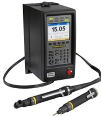
Figure 5.8: Electrical cord connects the tool with the controller
