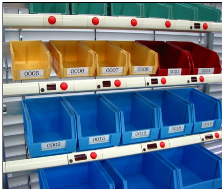
Figure 5.65: Pick-to-light error-proofing system
