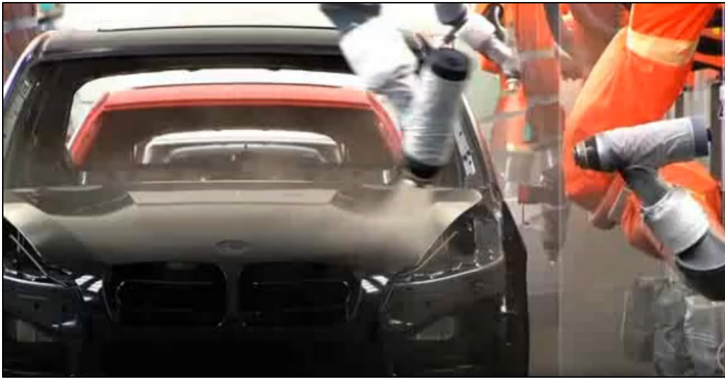
Figure 2.3: Car body being painted by robots in a Paint Booth
