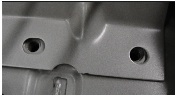
Figure 4.7: Assembly sequence driven by locating hole
