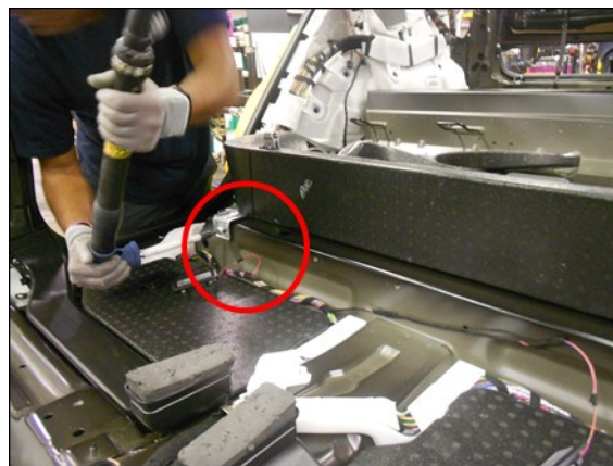
Figure 6.2: Seat Adapter assembly process
