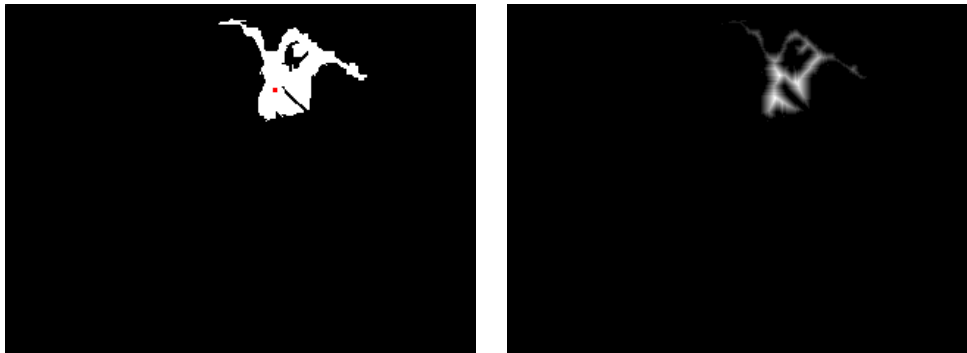
Figure 3.4: LEFT: The binary region associated with an article of clothing (orange shirt), with the grasp point (red dot) computed as the location that maximizes the chamfer distance. RIGHT: The chamfer distance of each interior point to the clothing boundary.
