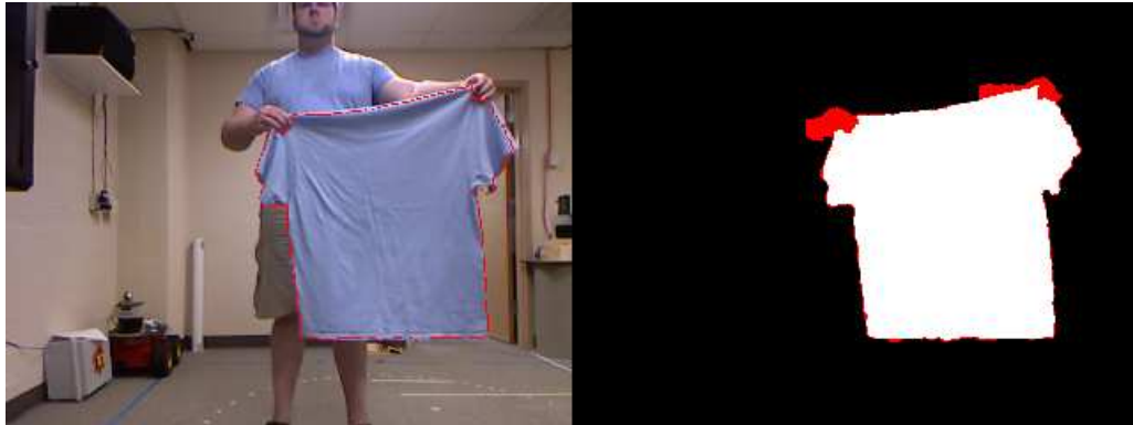
Figure 5.7: Left: Color image within a shirt sequence. Right: Segmentation of shirt from background while using the skin detector. White pixels represent foreground (shirt), black pixels represent background, and red pixels represent skin.
