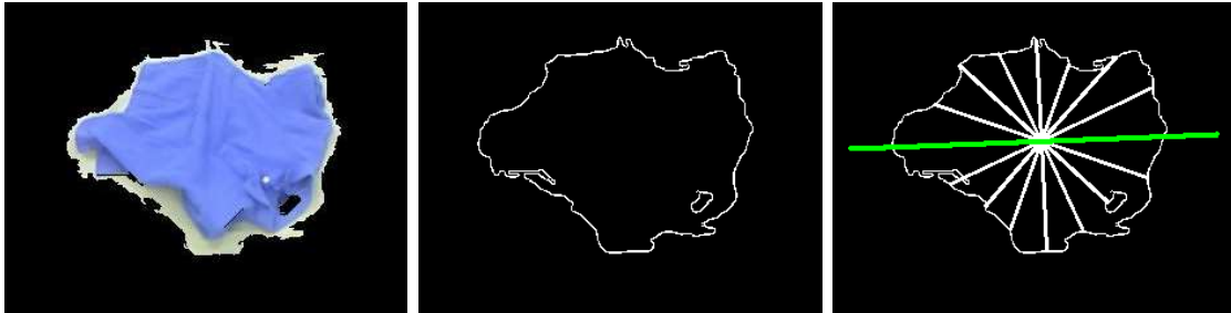
Figure 3.15: LEFT: Article segmented from background. MIDDLE: The binary boundary of the article. RIGHT: The boundary of the article along with the lines connecting the centroid to the boundary, whose distances are used in the feature vector. The green line represents the major axis found by PCA.
