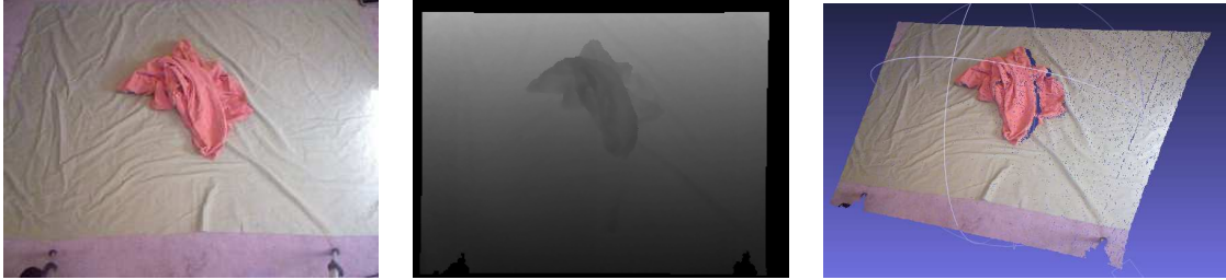
Figure 3.8: Data to be used in my approach. From left to right: Color image, depth image, and a point cloud of a t-shirt.
