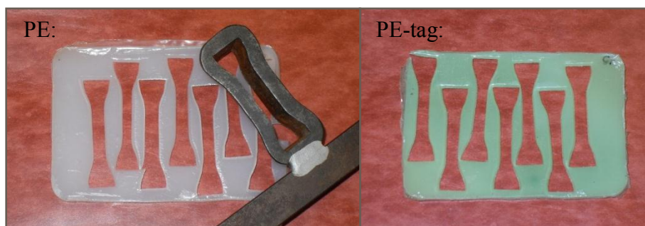
Figure 2.2: Dogbone die and sample blocks from which specimens were cut for tensile testing
