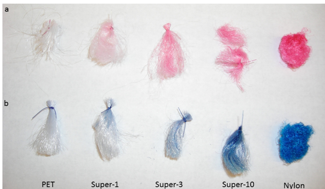
Figure 3.6. a) C-CP fibers (PET, Super-1, Super-3, Super-10, Nylon) dyed with C.I. acid red 1 to visually reflect the anionic functional groups. b) C-CP fibers (PET, Super-1, Super-3, Super-10, Nylon) dyed with methylene blue (basic blue 9) to visually reflect the cationic functional groups
