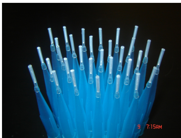
Figure 2.3. Photograph of C-CP fiber packed SPE tip attached to micropipette tip
