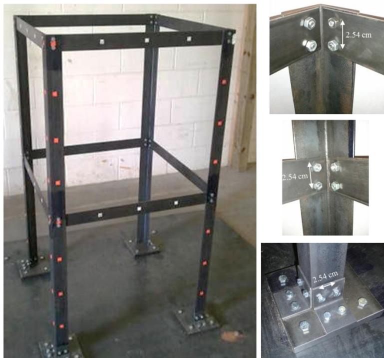
Figure 5.4: Frame structure built in the laboratory (Left) and frame connections (Right): Top connection (Top), Middle connection (Middle), Base connection (Bottom).
