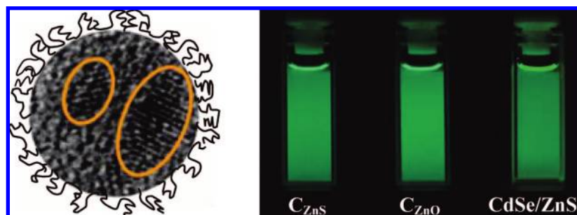
Figure 1. Left: cartoon illustration on carbon dots with a doped carbon core (from an experimental HR-TEM image with ZnS lattice fringes circled). Right: aqueous solutions of C_{ZnS} -Dots and C_{ZnO} -Dots (450 nm excitation for both) compared with a commercial toluene solution of CdSe/ZnS dots (matching optical density at excitation), all photographed through a 475 nm cutoff filter.
