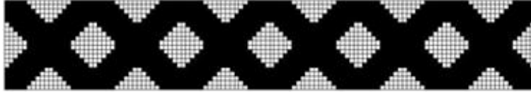
Figure 1.11: Example of a meta-material that violates the homogenization limit in the vertical direction (and likely the horizontal direction).
