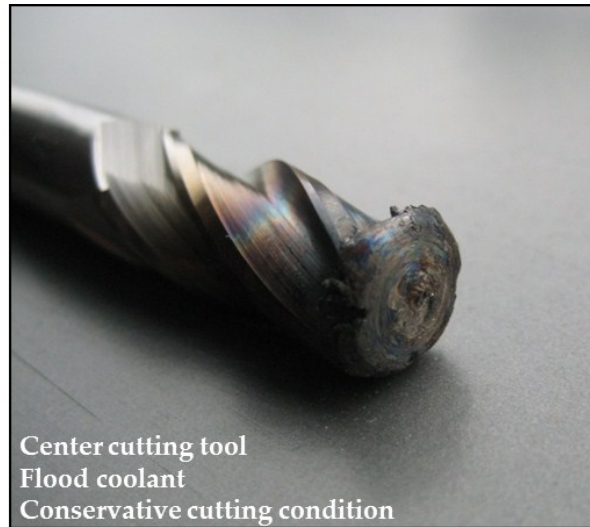
Figure 1-1: Catastrophic failure of a NIAGARA high-performance solid-carbide end mill. This center-cutting tool failed a few minutes into milling Ti-6Al-4V when roughing the bottom of a drill hole. Note the discoloration due to overheating half-way up the cutting flutes. The other main cause was the retained high-temperature strength of Ti-6Al-4V, leading to welding and smearing of the tool (5-flute, TiAlN coated, \phi 0.5'' end-mill), (Cost: $63.70 from Travers, Inc.).
