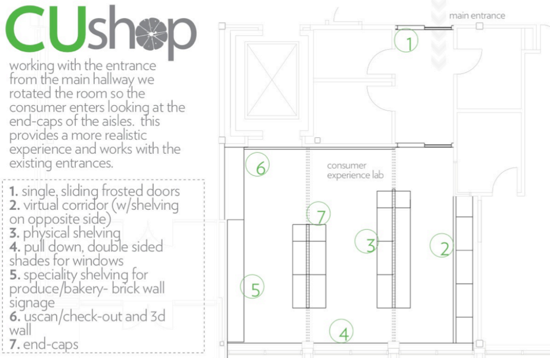
Figure 4.10: Shop Specification in Existing Room
