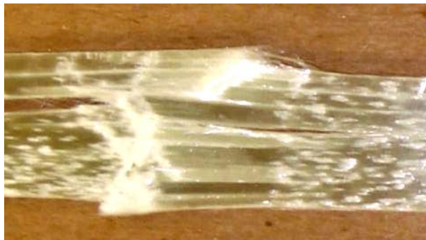
Figure 4.14: Laminate composite specimen after ASTM D6641 testing. Measured compressive strength was 0.56 MPa
