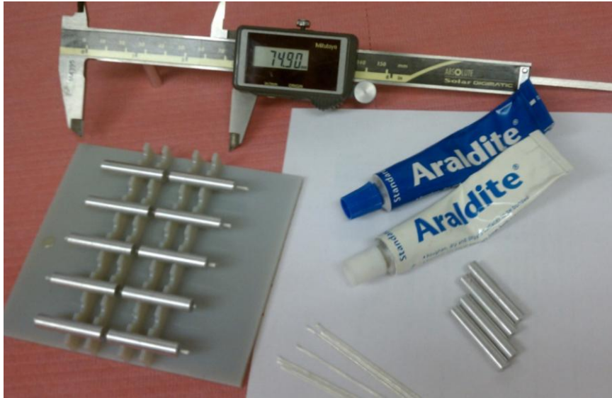
Figure 4.9: Monofilament samples, aluminum cylinders, epoxy, and digital ruler used in sample construction
