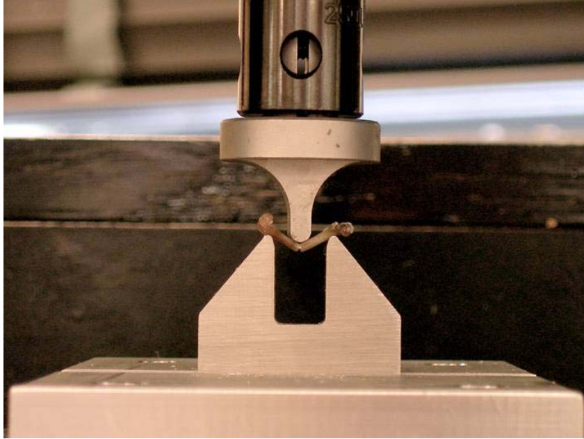
Figure 3.4 Three point bending test on mid-femur with 8 mm span length
