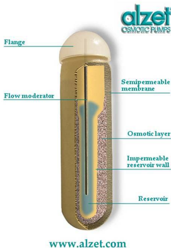
Figure 4.2 Diagram of Alzet osmotic pumps for drug delivery
