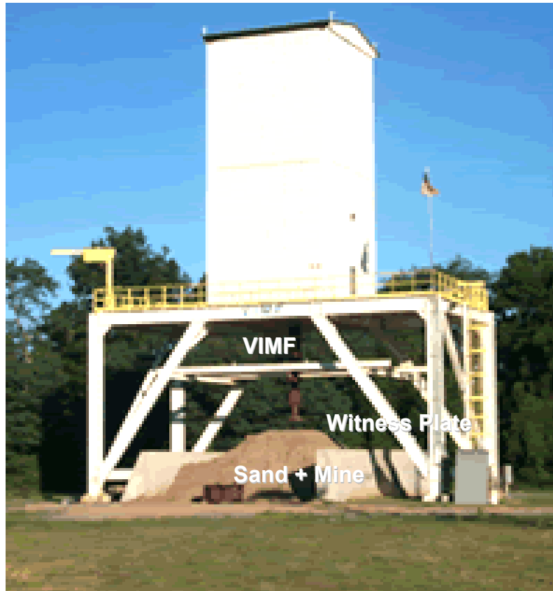
Figure 3-8. Vertical Impulse Measurement Fixture used in Ref [3.15]
