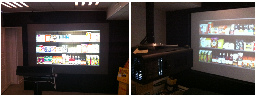
Figure 2.4: The Packaging Arena media lab utilizing rear projected images (note the space required behind the screen).
