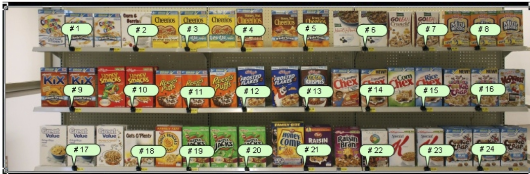
Figure 3.11: Still image of shelf with IR markers that are used to map the physical space to the image space.
