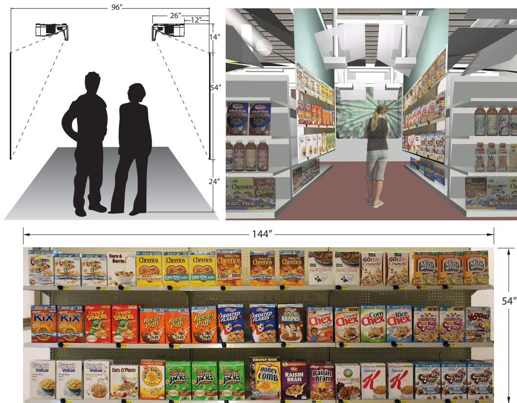
Figure 5.7: Virtual aisle provides life-sized projected image that fills peripheral vision and allows close proximity to screens without shadow interference.
