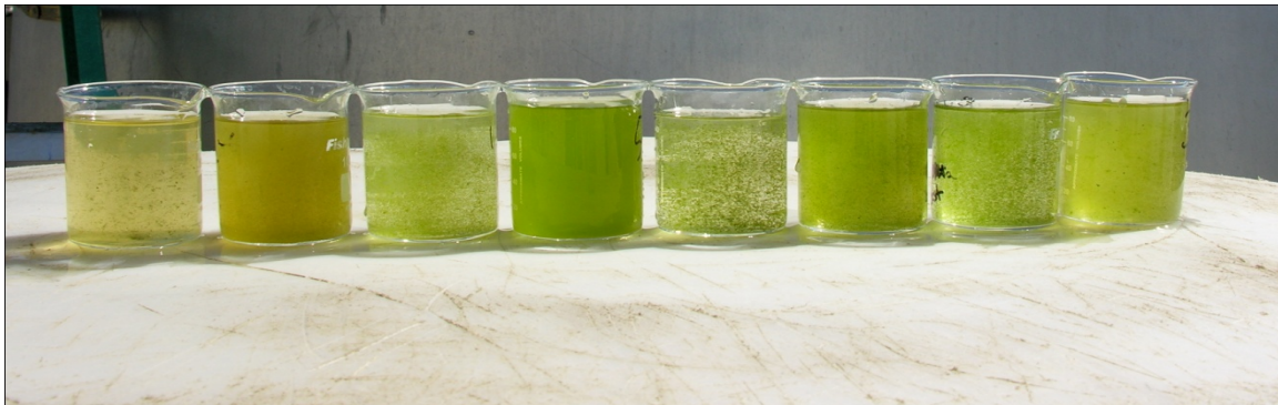
Figure 57: Pilot plant algal post treatment at landfill site II beginning of March 2010, Unit #1 through #8 (from left to right); directly after sampling (Kent Bioenergy).
