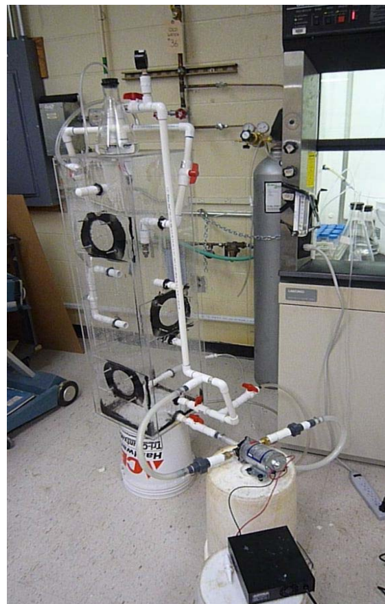
Figure 3: Laboratory absorption column with acid recycle pump, spray nozzles from top, acid trap on top.
