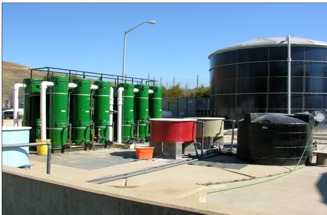
Figure 7: Ammonia Recovery Process at "landfill site II", showing green de-sorption and absorption columns on the left and the blue leachate storage tank in the back.
