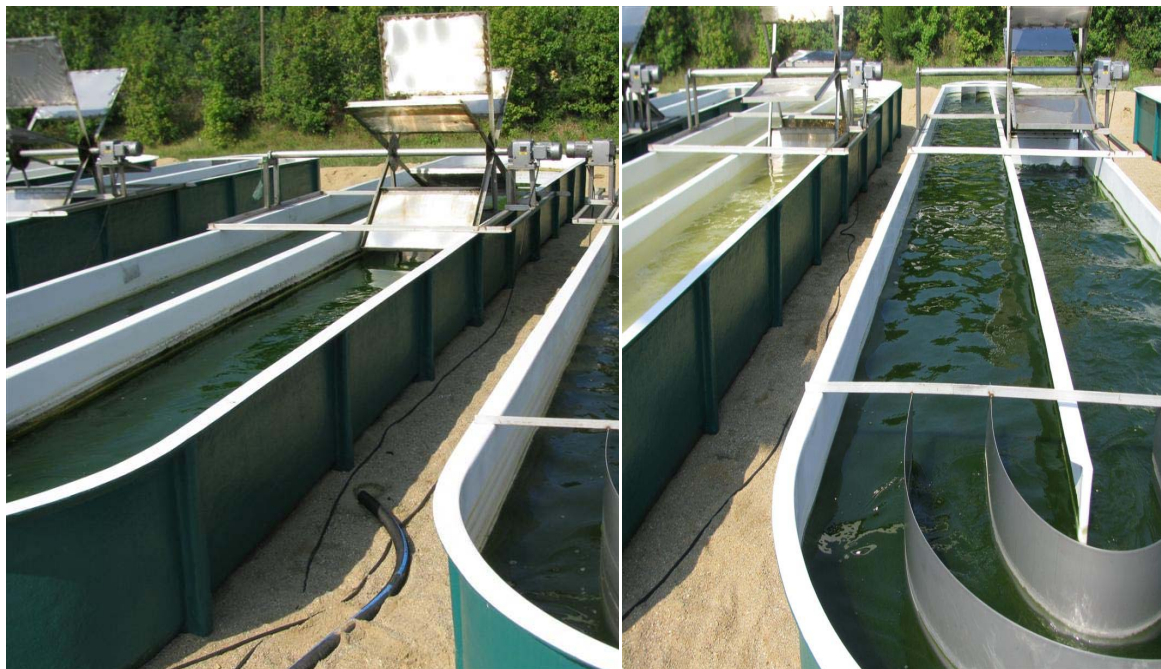
Figure 15: Pilot plant high-rate algal post treatment units operated by Kent Bioenergy located at landfill site II.
