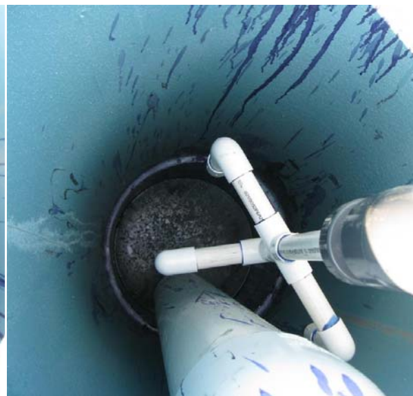
Figure 10: Internal view of de-sorption column showing spray nozzles.
