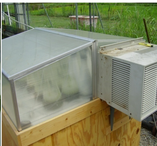
Figure 14: Temperature controlled algal culture apparatus with A/C unit.
