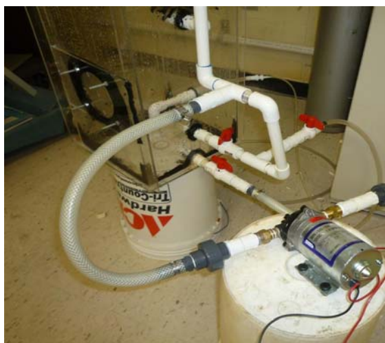
Figure 4: Laboratory absorption column with acid recycle pump, gas inlet on bottom.
