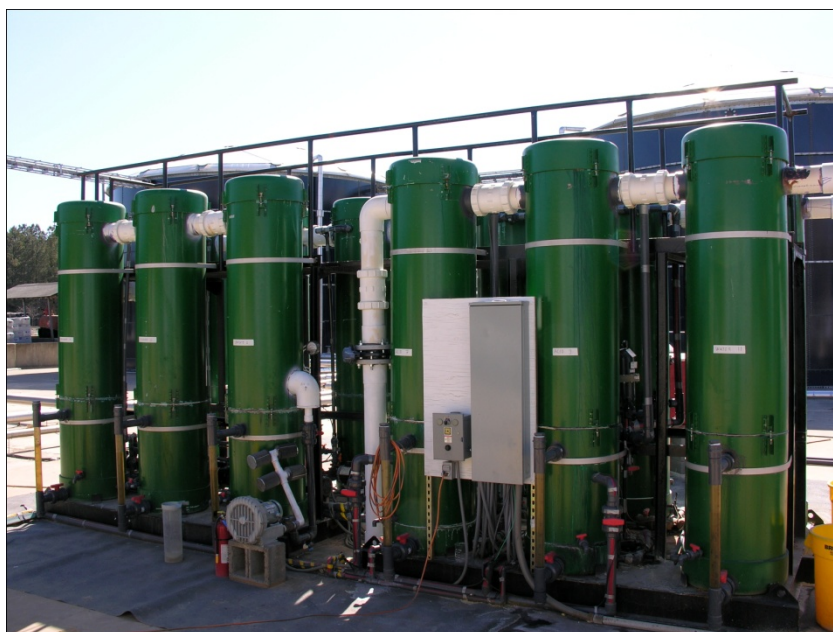
Figure 7: Ammonia Recovery Process at "landfill site II", showing green de-sorption and absorption columns on the left and the blue leachate storage tank in the back.
