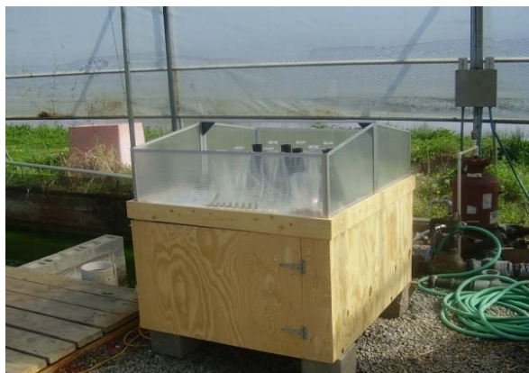
Figure 61: Algal culture apparatus.
