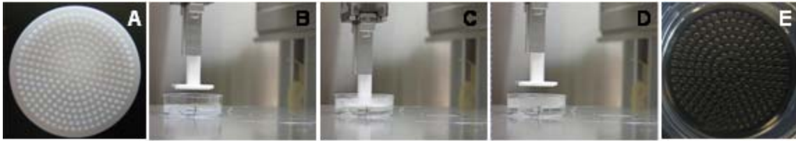
Figure 5. 2: (A) Plastic male-mold used to fabricate agarose microwells, (B-D) automated robotic stamping of agarose gel by the plastic male-mold, and thus (E) robotically produced agarose microwells.
