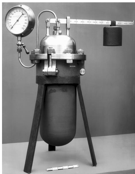
Figure 1.2. Papin's digester as made for laboratory use. Adapted from
