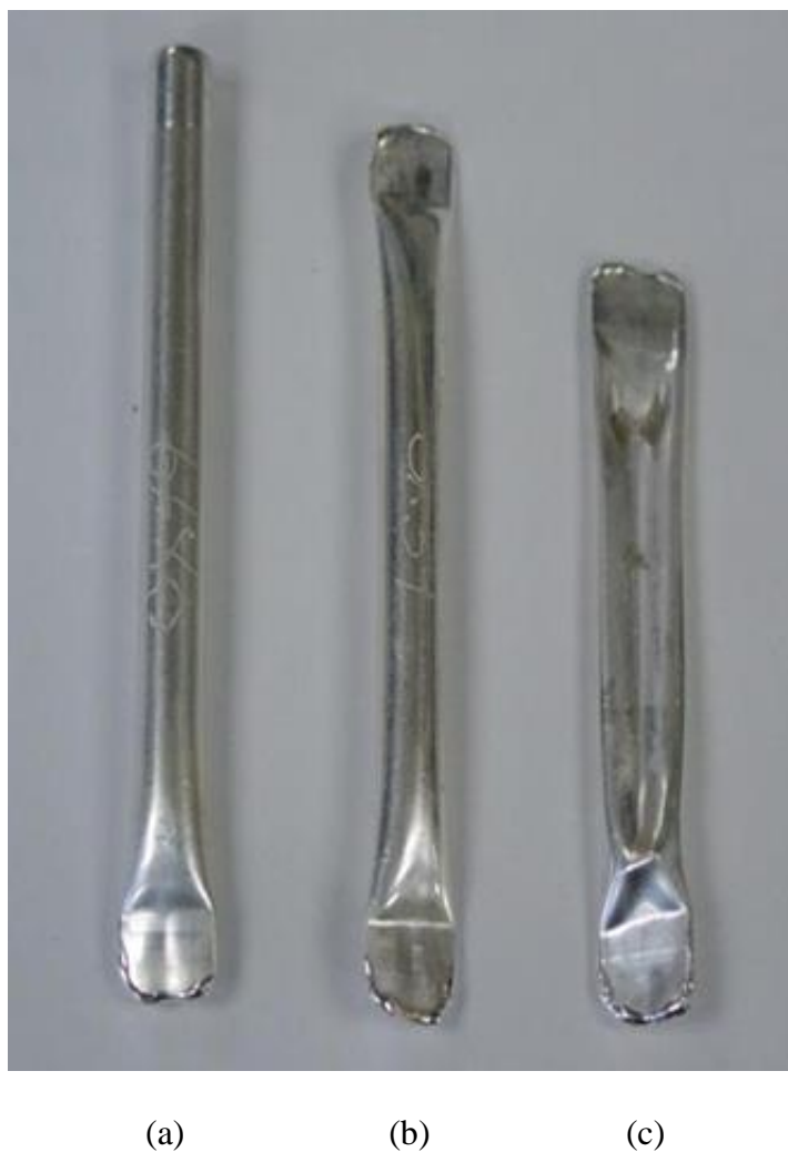
Figure 2.1. Progressive steps to sealing a silver ampoule. (a) One end welded, ready for sample charging. (b) Fully welded sample ready for hydrothermal treatment. (c) Ampoule after hydrothermal treatment.
