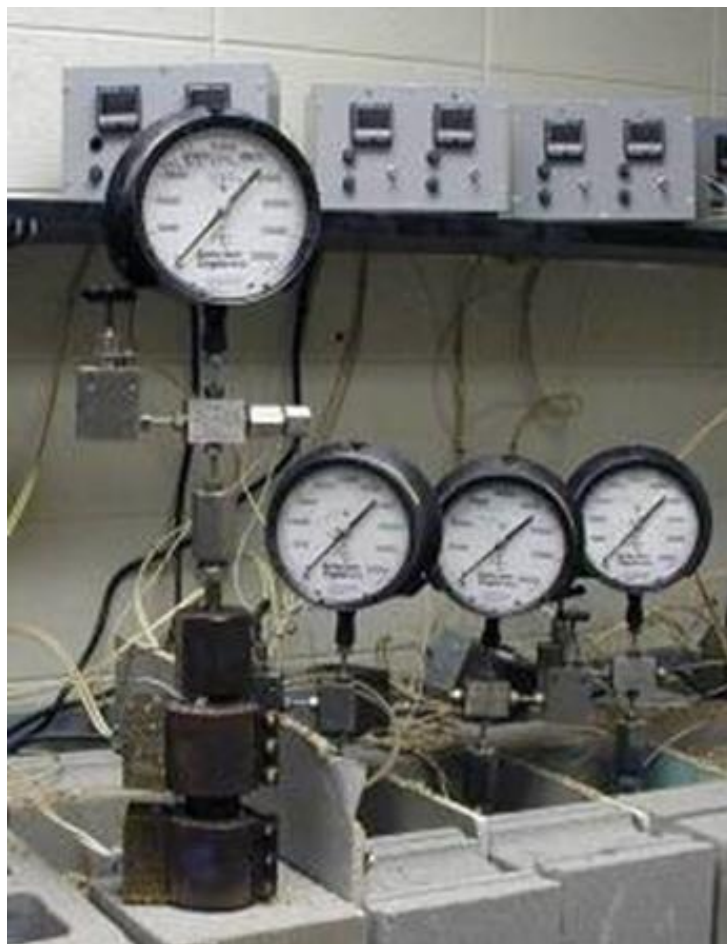
Figure 2.2. Typical full setup of a floating-liner autoclave, complete with band heaters and cinder block pits.
