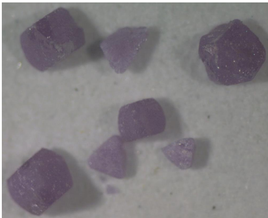
Figure 7.2. Photo depicting the trigonal prismatic and polyhedral morphologies of \text{Na}_3\text{Nd}_9\text{B}_8\text{O}_{27} .
