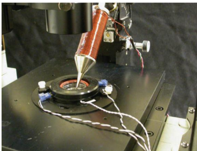
Figure 3.6. Magnetic trap for high force cell probing, composed of electromagnet with sharp tip on a micromanipulator. Imaging is performed on a microscope stage with a stage heater to maintain physiologically relevant temperatures [30].
