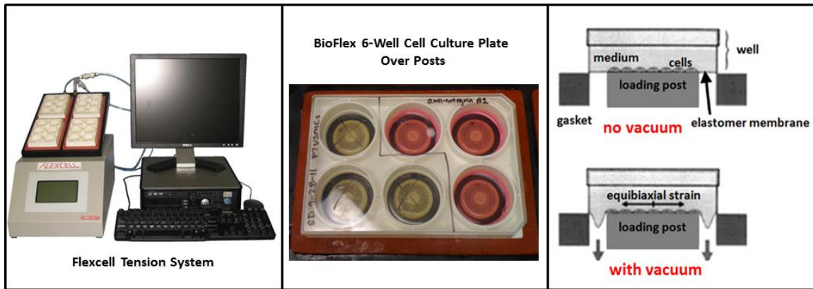
Figure 7.2. Flexcell Tension System. A computer-regulated bioreactor (left) uses vacuum pressure to apply cyclic strain to cells (right) cultured on flexible-bottomed culture plates (center) [14, 15].
