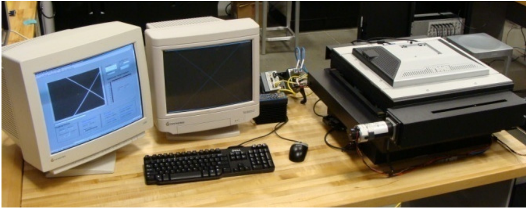
Figure 3-2: Direct Position Sensing's prototype. The prototype configuration of Direct Position Sensing where the LCD screen is located on top of a XY table for target display and tracking purposes
