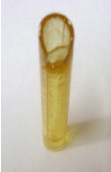
Figure III.23: Picture of "Hollow Tube" of 70\text{TeO}_2\text{-}10\text{Bi}_2\text{O}_3\text{-}20\text{ZnO} glass
