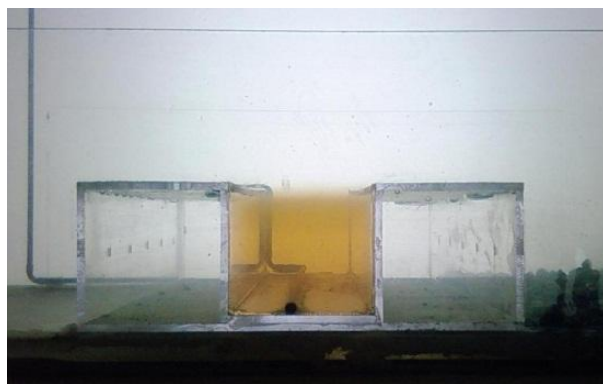
Figure 2.8: The flooded flume with the canyon space full of dyed saltwater.
