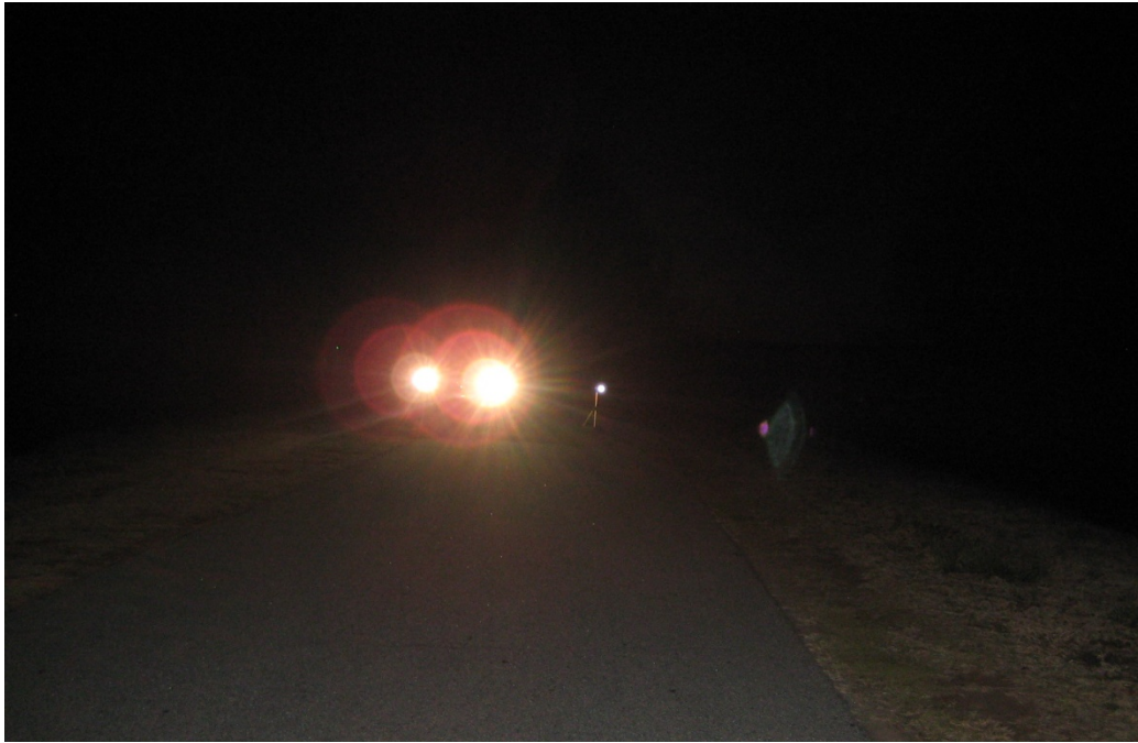
Figure 19. Position of the Landolt C stimulus in relation to the glare source vehicle. Both the glare source vehicle and the participant vehicle have high beam headlights turned on. The camera flash was not used.
