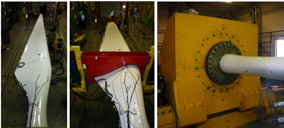
Figure 4.2: Experimental fixed-free (left) configuration, mass-added (middle) configuration, and base fixture (right).
