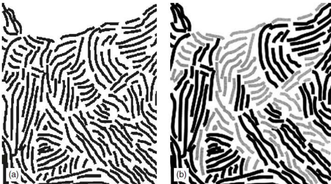
Fig. 1.6 The Norit model: (a) structure before activation; (b) removal of some of the graphene layers (as indicated by the lighter color) either individually or in groups as a result of activation. (Reprinted with permission from Marsh and Reinoso, 2006. Copyright 2006 Elsevier.)
