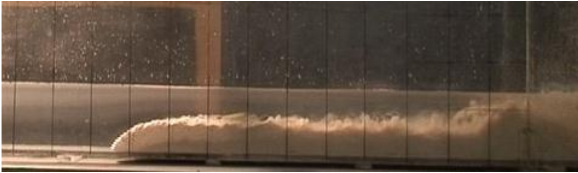
Figure 3.2. Propagation of the constant-volume released fluid mud underflow in Exp. # 5 after 9 seconds of releasing the fluid mud suspension in a rectangular flume. The current front position, x_N , is at 102 cm from the lock-gate at the shown instant.
