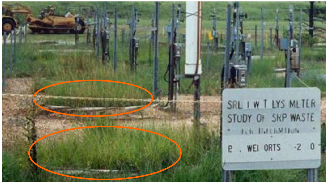
Figure 2.4 A photograph of the SRS lysimeter study area shows grass plants growing in and around the highlighted lysimeter surfaces.
