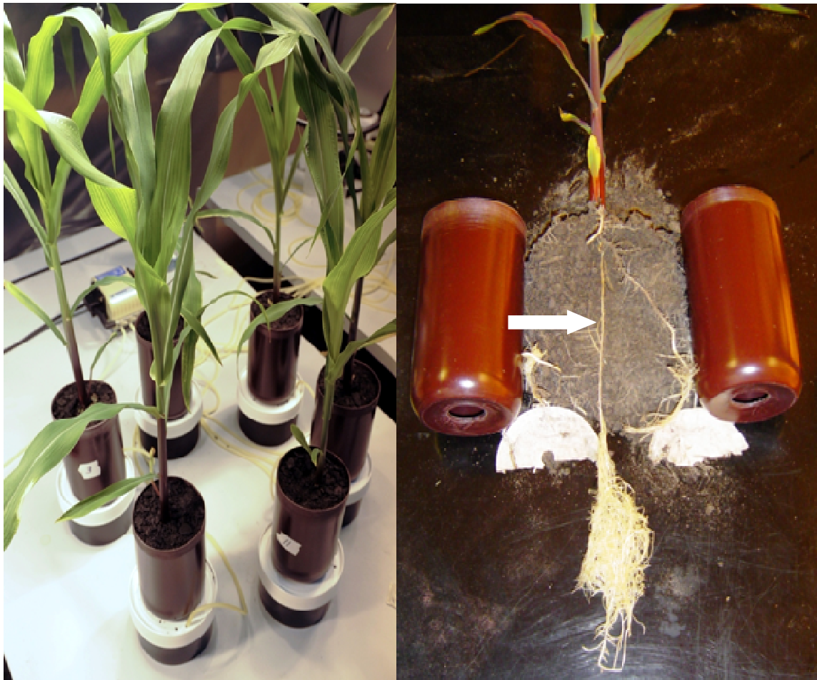
Figure 5.1 Corn plants growing in soil pots with the primary root inserted in nutrient solution. On the left, corn grown under plant lights; on the right, with the soil and nutrient pots removed, the primary root is exposed. To initiate an experiment, complexed Pu was added to the hydroponic solution.
