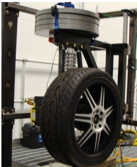
Figure 7-1 DEEDS prototype hardware installed on a single post shaker
