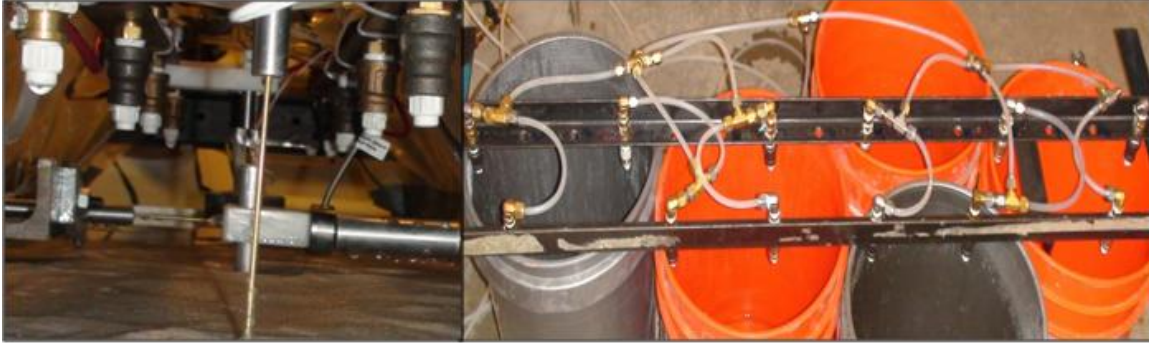
Figure 10.19 The nozzle system with equally distributed tubing
