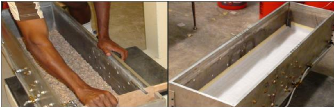
Figure 10.4 The container with the drainage layer
