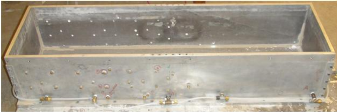
Figure 10.3 The container with drainage tube system
