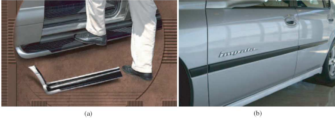
Figure 1.2: Application of nanocomposites in automotive parts [13]: (a) M-Van step Assist: 1st commercial launch. (b) Impala: 2nd nanocomposite application.
