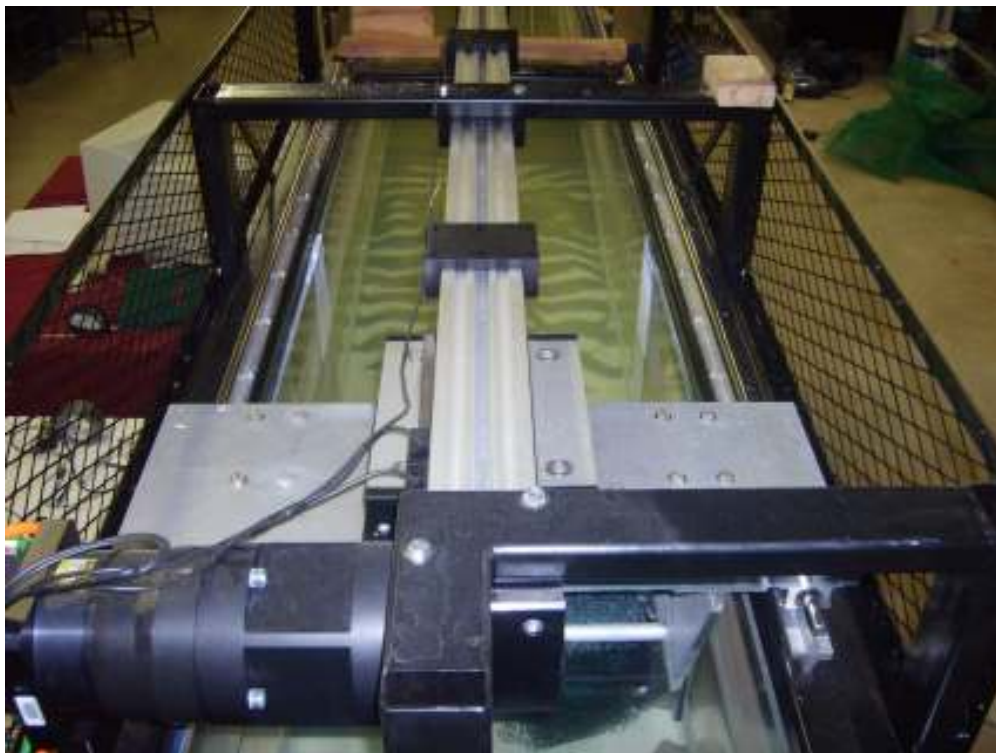
Figure 3.2 Piston-type wavemaker at Flow Physics Laboratory of Clemson University
