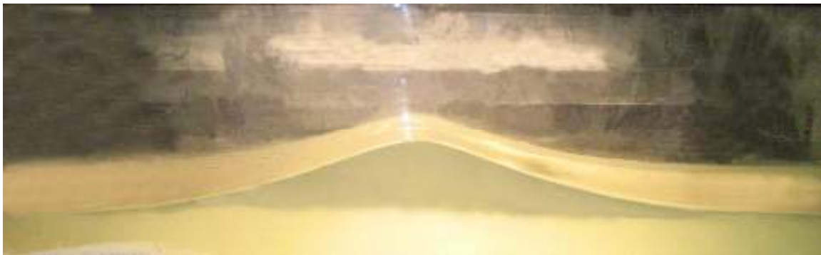
Figure 4.3 Photograph of a typical solitary wave generated in the wave-tank. Rayleigh-type solitary wave generated by the New methodology for \varepsilon = 0.6 in still water depth of h = 20\text{ cm} . Photographed at 15h from the wave paddle.
