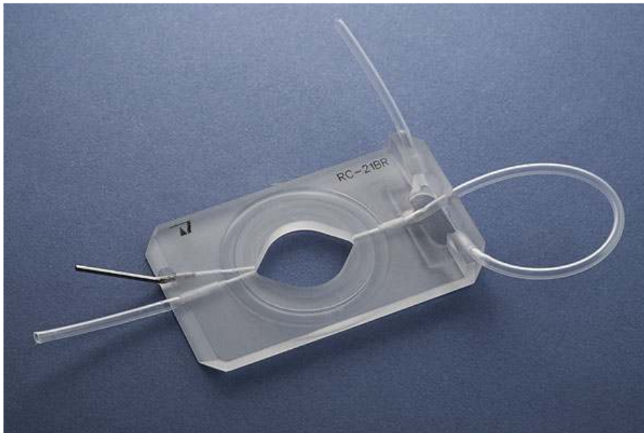
Figure A-2: Assembled view of Warner RC-21 chamber
