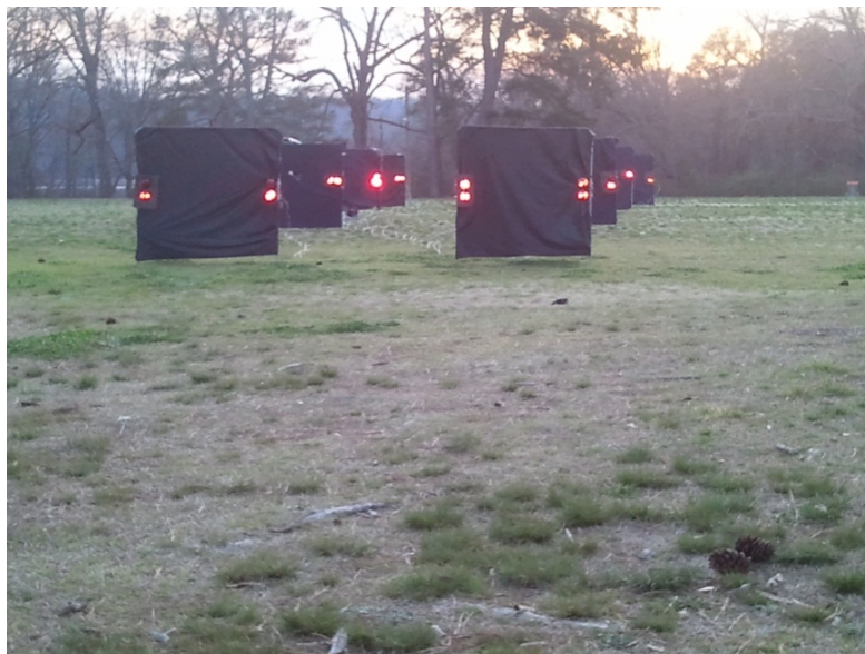
Figure 5.2. Eight vehicle display in Red condition with brake lamp activated in left lane third row.
