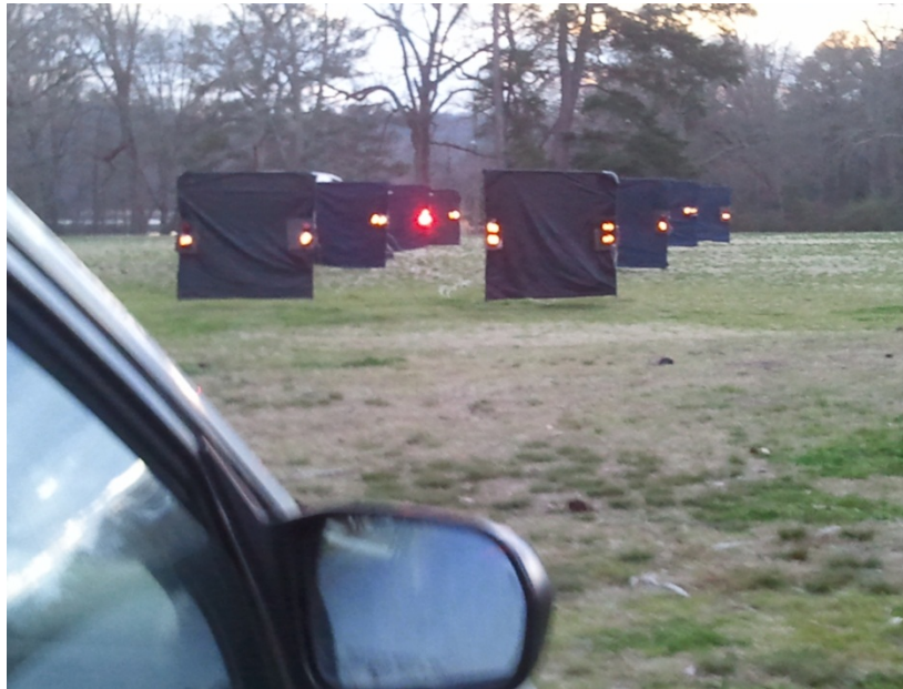
Figure 5.1. Eight vehicle display in Amber DOT condition with brake lamp activated in left lane third row.
