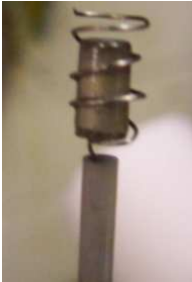
Figure 3.3 The specimen holder for the oil-quench furnace.
