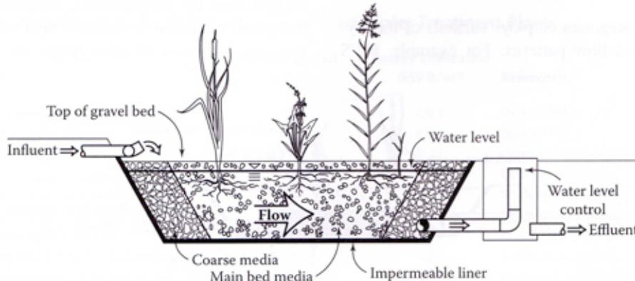
surface of the media to prevent exposure to humans or wildlife. Subsurface flow CWs can be operated in continuous-flow or batch-load treatment modes with varying hydraulic residence times (Burgoon et al., 1995). Pretreated wastewater flows by gravity, horizontally or vertically, through the bed substrate where it contacts a mixture of facultative microbes living in association with the substrate and plant roots. The majority
