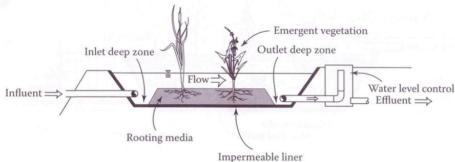
a concomitant increase in depth (~1.25-1.5 m), which promotes anaerobic conditions that facilitate denitrification. The large land area required by typical SF constructed wetlands and the concomitant loss of production area has made them less attractive for greenhouse and nursery water treatment than SSF CWs ( Berghage et al., 1999).
