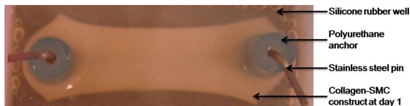
Figure 3.1: Statically loaded RASMC-seeded 3-D collagen gels. Gels, shown at day one of culture, were cast within silicone wells and anchored to polyurethane end-holders
