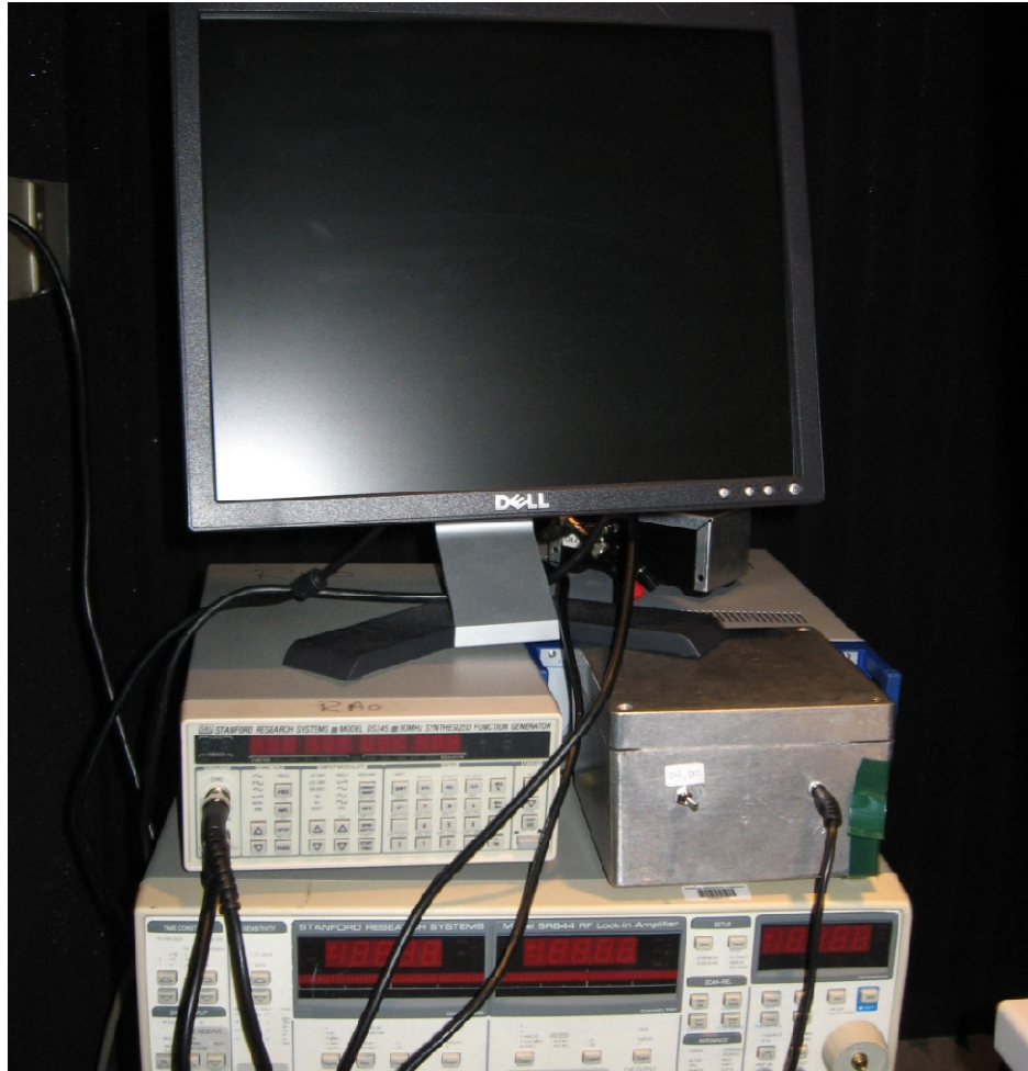
Figure B-3: External electrical setup for HDR experiments under vacuum. From top: monitor for use with controlling PC (not pictured) and dc bias unit, function generator and preamplifier power supply, lock-in amplifier.
