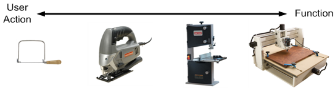
Figure 8-2: Example of Solutions to Wood-Cutting Problem on a Function-User Continuum (image sources, left to right: sears.com, sears.com, sears.com, rockler.com)
