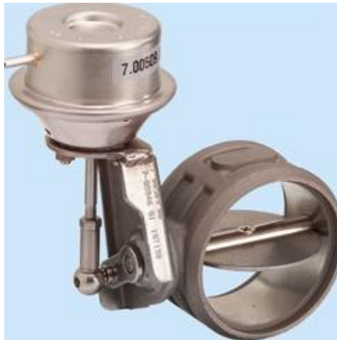
Figure 8.1: Pierburg Exhaust Gas Bypass Flap [192]
