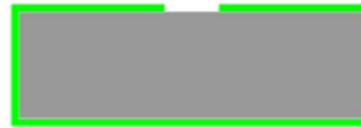
(e). Strip off photoresist
