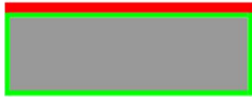
(b). Photoresist spun
