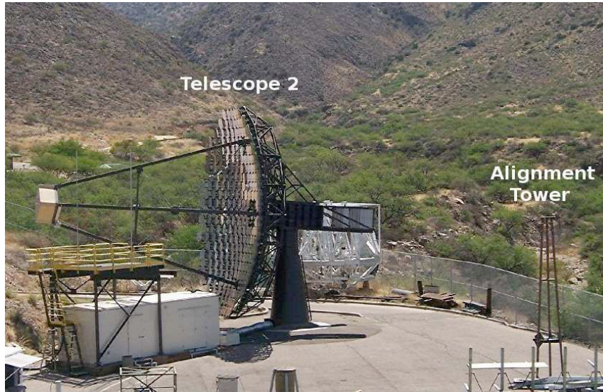
Figure B.2 Telescope 2 and its Alignment Tower, located at the “ 2f ” point. Image taken from [Toner et al. 2008].
