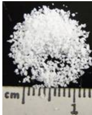
Figure 5.1: Ceramic Granules. The \beta -tricalcium phosphate ceramic granules of bone void filler, 0.5 - 0.7 mm in size were used in this study (Synthes, USA; Paoli, PA).
