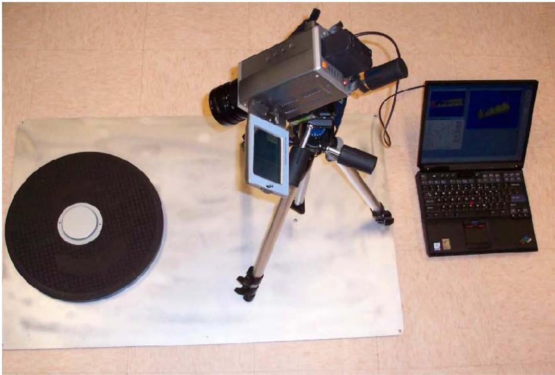
Figure 2.11: The Thermal Distribution Acquisition System
