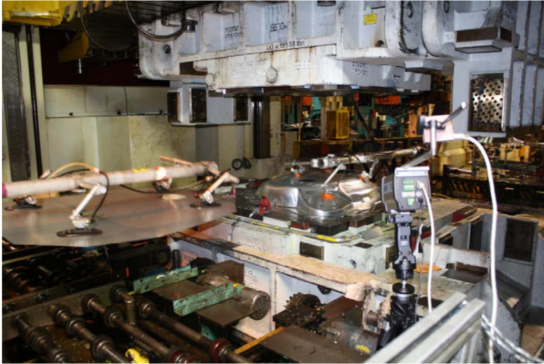
Figure 5.2: Experimental Setup of PCA based Image Fusion System
