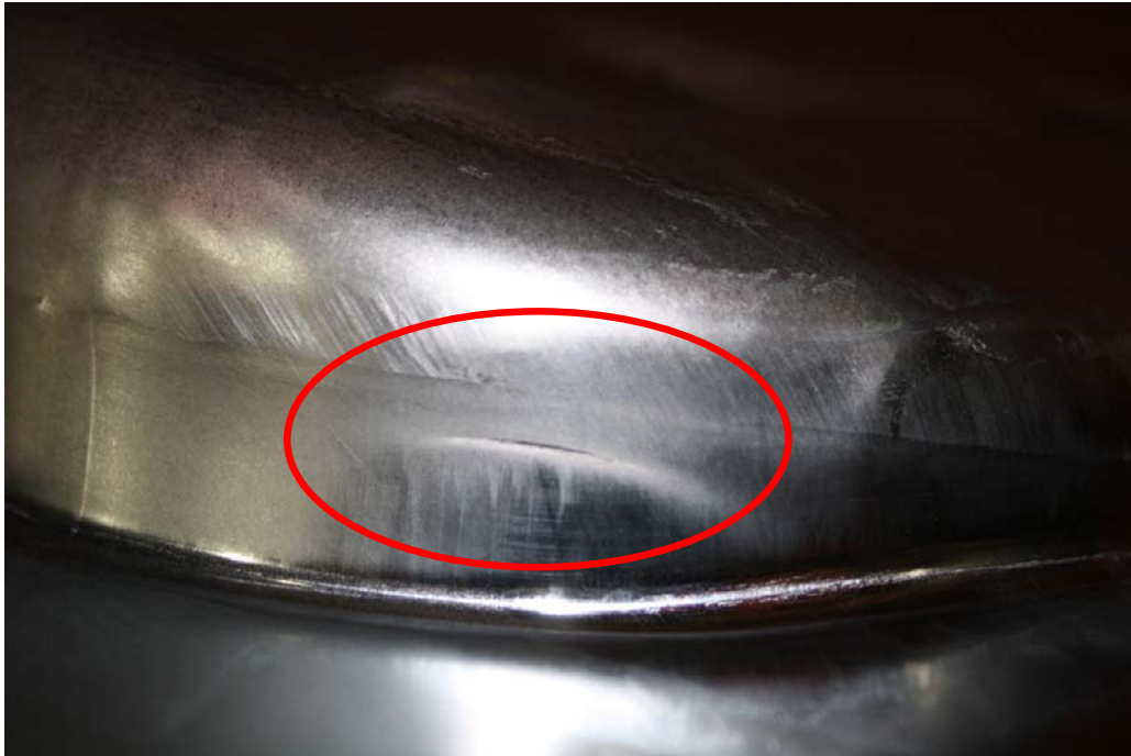
Figure 5.3: Stamping Split Sample of Vehicle Wheelhouse Part
