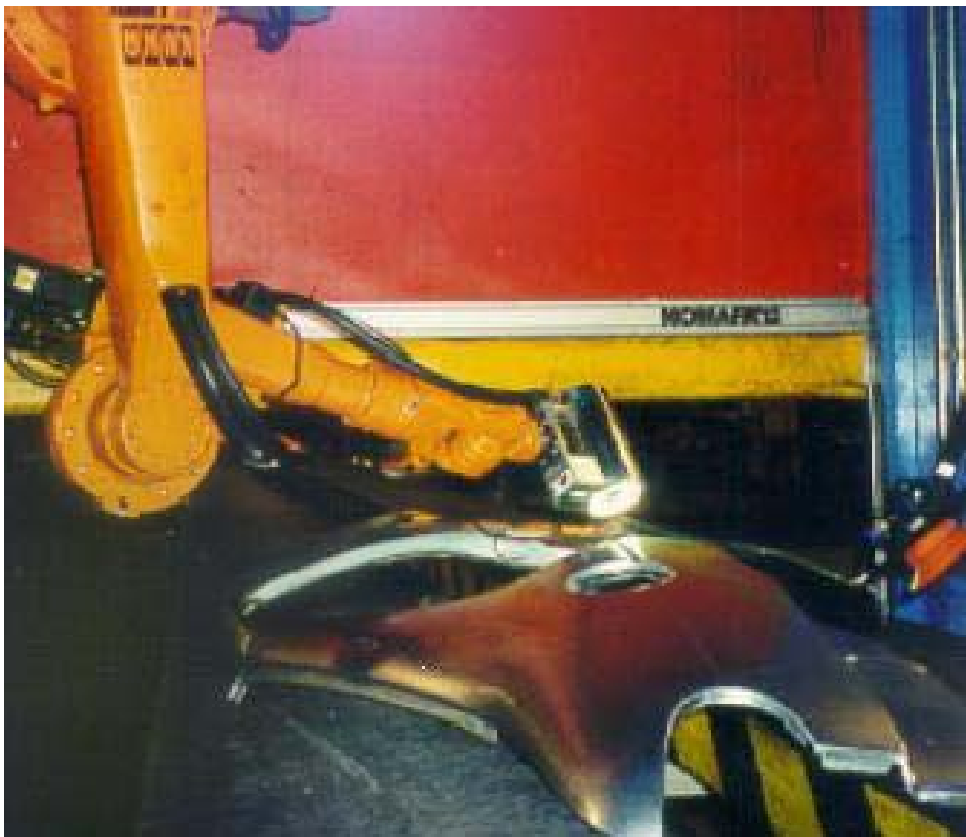
Figure 2.9: The Automatic Inspection System for Flow Detection on Car-body Parts
