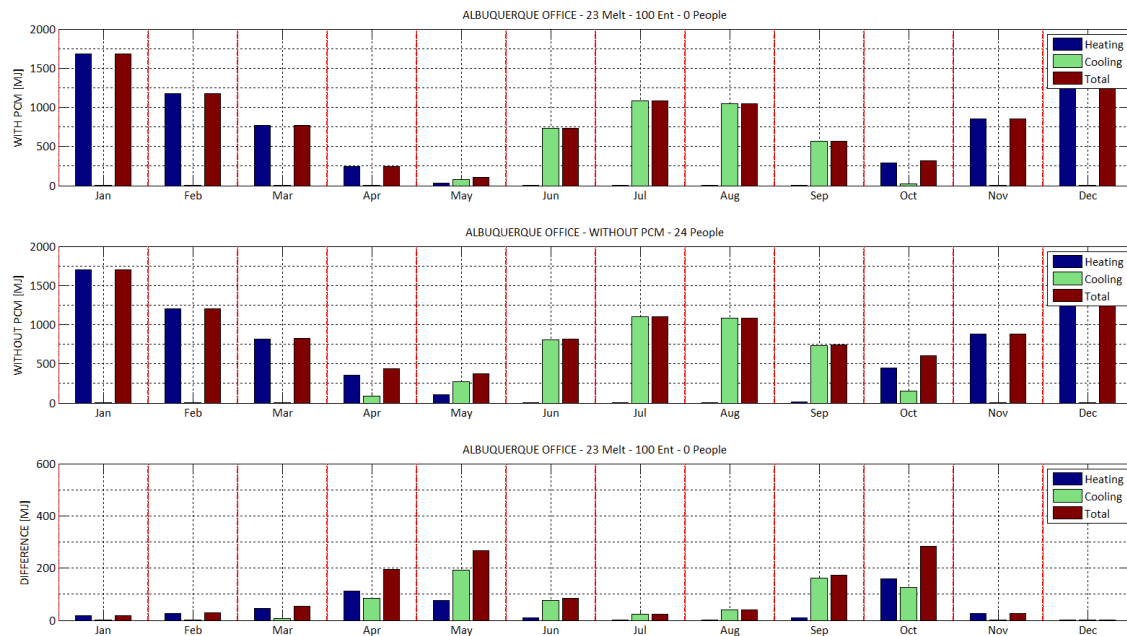
Figure 8.6: Albuquerque - office HVAC – 23-100-PCM - 0 people - monthly loads. With PCM (top) without PCM (Middle), magnitude energy saved (bottom).
