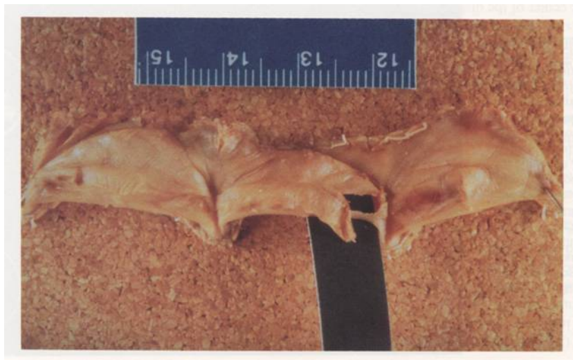
Figure 2.24: Structurally damaged bioprosthetic heart valve
