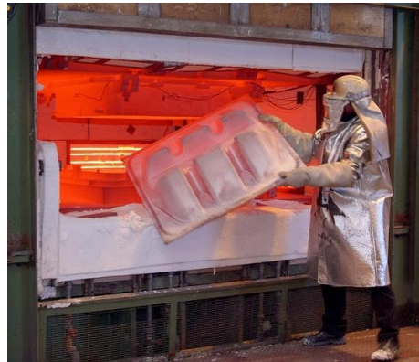
Figure 7. Superplastic forming [25]. A part is heated to roughly two-thirds of its melting temperature and formed to allow for great elongations and a formed part with very few residual stresses.
