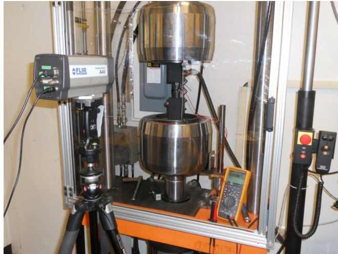
Figure 92. Experimental test setup for contact area effect investigation. This testing setup includes a multi-meter that reads the voltage drop across the top and bottom dies at the locations where they contact the test specimen.
