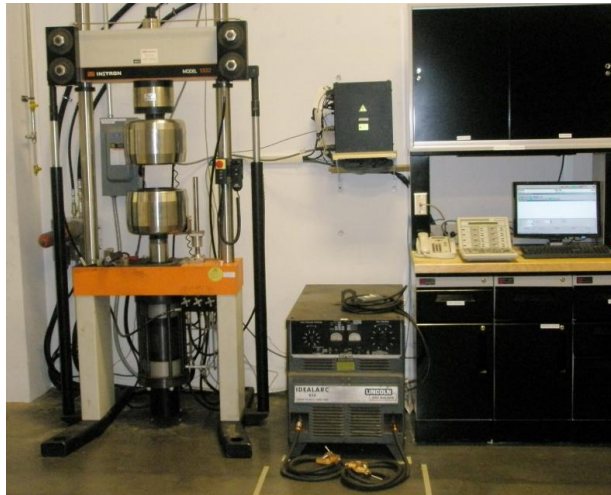
Figure 191. Instron EAM testing setup at CU-ICAR. The EAM testing setup includes an Instron hydraulic testing machine, a controllable DAQ, and a power supply.
