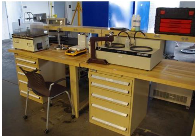
Figure 192. Microstructure sample preparation cell. The microstructure setup includes a cut-off saw, mounting supplies, and a dual-table grinding/polishing station for preparation of microstructure samples.
