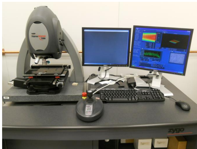
Figure 85. Surface roughness measuring equipment. A Zygo New View 7200 optical surface profilometer equipped with MetroPro analysis software was used to determine the surface roughness of the specimens.
